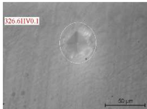
Figure IV.8 – Enamel indent, Group 1 - sample M 1A la pH 6.5 (Time = 10s, Load= 100gf).
