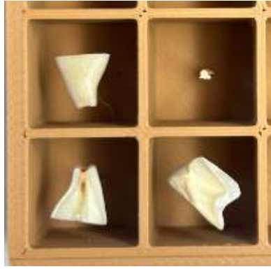
Figure V.9 – lengthwise and crosswise sections of teeth samples to expose the enamel for further hardness testing after exposure tooo welding fumes
