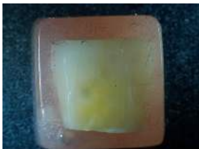
Figure VI.13 - Illustrations of dental enamel samples fixed in acrylic resin after the 36 hour and 48 hour exposures to 65 % HNO 3 , prepared for hardness testing
