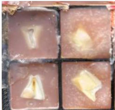
Figure V.12 – Fixed enamel samples in acrylic resin
