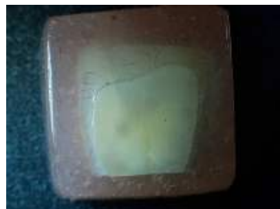
Figure VI.13 - Illustrations of dental enamel samples fixed in acrylic resin after the 36 hour and 48 hour exposures to 65 % HNO 3 , prepared for hardness testing
