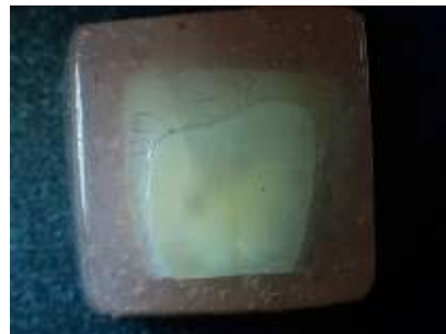
Figure VI.12 – Illustrations of dental enamel samples fixed in acrylic resin after the 12 hour and 24 hour exposures to 65% HNO 3 , prepared for hardness testing
