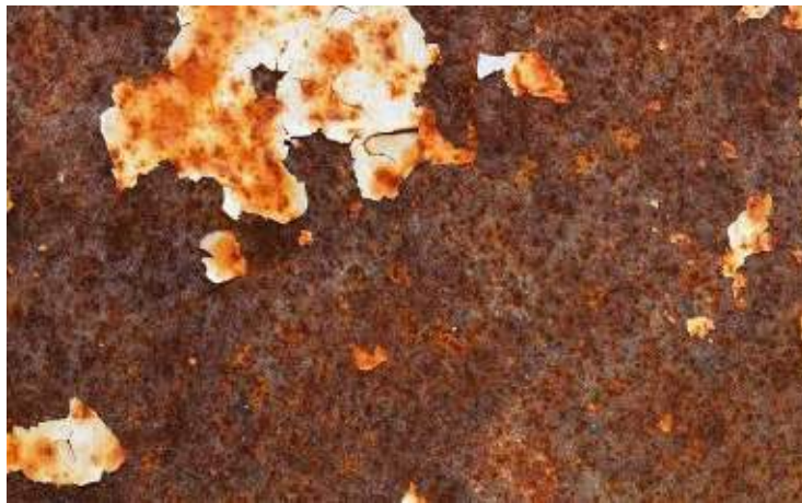
Fig 6.11 Uniform corrosion - tank
