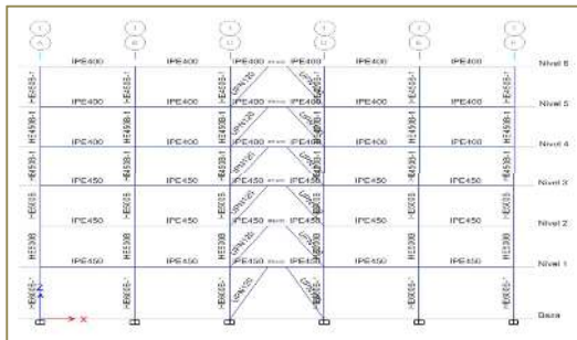
Figure 5.2.3 Eccentric brace structure (SMCE)
