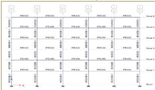
Figure 5.2.1 Unbraced structure (SMNC)
