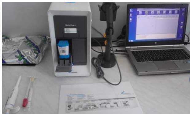
Fig. 9. GeneXpert Instrument Systems (GeneXpert apparatus, barcode scanner, GeneXpert computer software, user manual, stick and mixer set, pipette)
