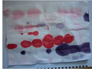
Figure 24 Appearance of blotting paper after successive absorption of fluids from the blade
