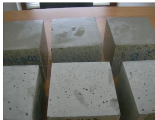
Figure 2.11-Comparisson between normal vibrated concrete porosity and self compacting concrete porosity- laboratory testing (author photo)
