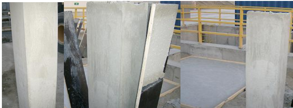
Figure 4.30,4.31,4.32- Precast self compacted concret elements after stripping (author photo)
