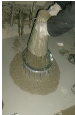
Figure 4.6-J- ring test for self compacted concrete
