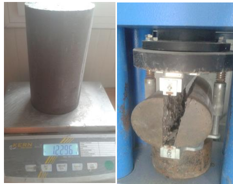
Figure 4.21, 4.22- Determining the resistance to splitting of SCC
