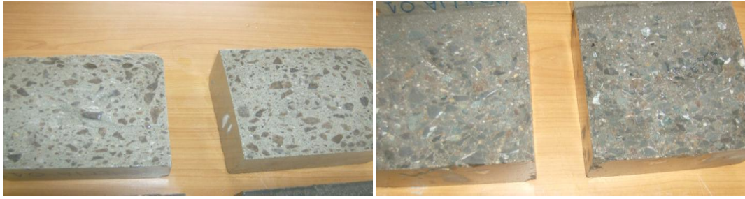
Figure 2.17, 2.18- Distribution of aggregates in self compacted concrete compared to normal vibrated concrete, laboratory test (author photo)
