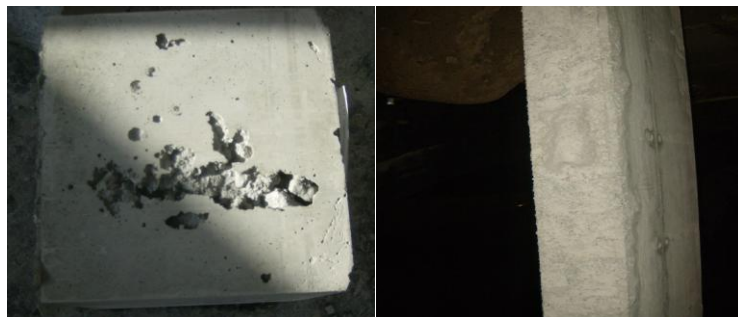
Figure 2.22, 2.23- Poor compacted concrete area: laboratory and construction site (author photo)
