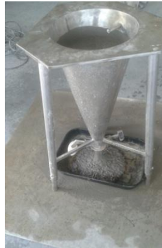
Figure 4.4- O'funnel test on self compacted concrete (author photo)
