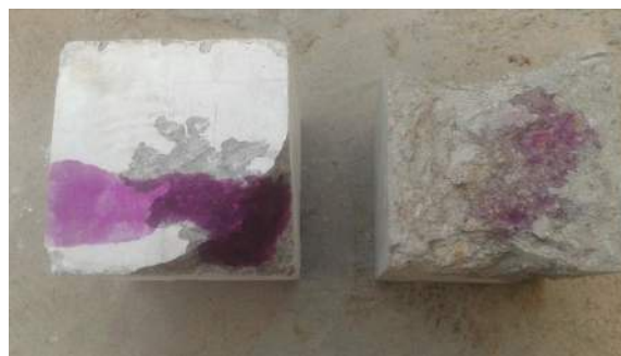
Figure 4.26- Highlighting the carbonation by treating the concrete crack with phenolphthaleine
