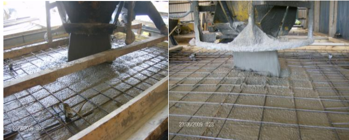
Figure 1.15, 1.16-Self compacted prefabricated factory, Leicester, Great Britain (author photo)
