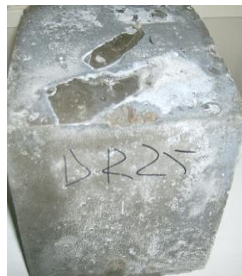
Figure 3.12- Concrete under sulphate attack, laboratory sample (author photo)
