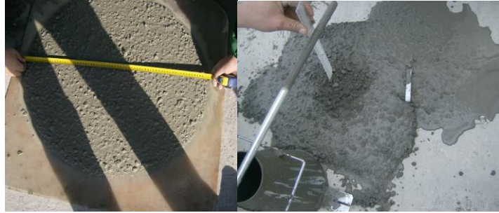
Figure 4.1, 4.2-Test for self compacted concrete spreading compared to subsidence to a fluid concrete (author photo)
