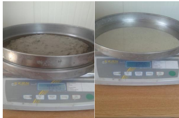
Figure 4.7, 4.8-Determinining the resistance to segregation using sieves
