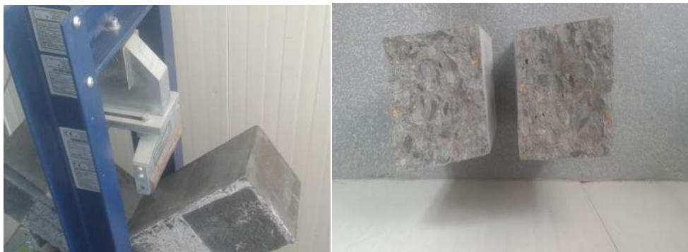
Figure 4.17, 4.18- Determinining the flexural tensile strength for SCC
