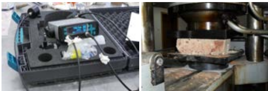
Fig. 4.29 - Trying destructive compression - (photo author)
