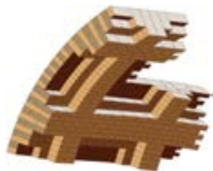
Fig. 2.51 - Weaving systems of masonry for vaults with large openings – (author drawing)
