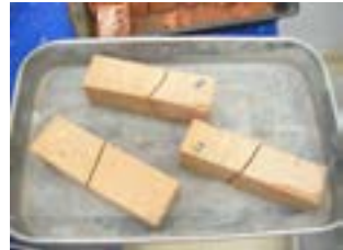
Fig. 5.52 – Brick samples tested for ultimate bending strength – (photo author)
