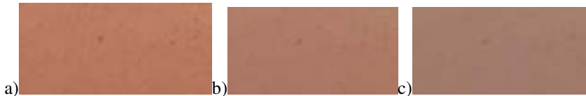
Fig. 5.65 - a) chromatic of the dried sample, b) chromatic of the treated sample with 10% consolidant, c) chromatic of treated sample 20% consolidant – (photo author)
