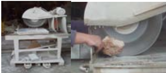
Fig. 3.23. Equipment used for cutting the stone blocks and making the samples
