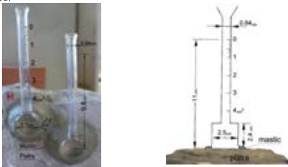
Fig. 3.37. Utilization of vertical Karsten tubes – dimensions
