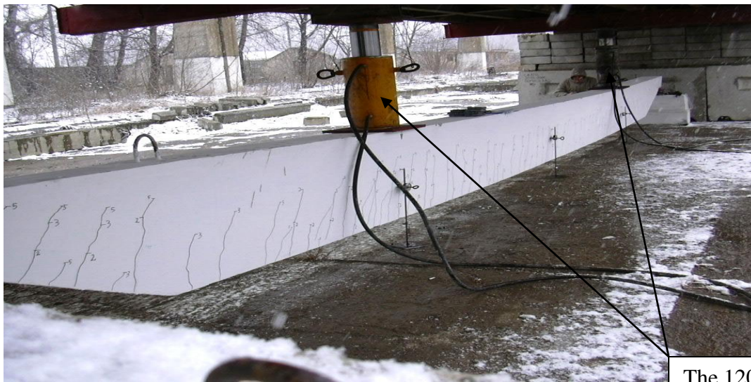
Fig. 3.20.-Testing the reinforced concrete roof beam
